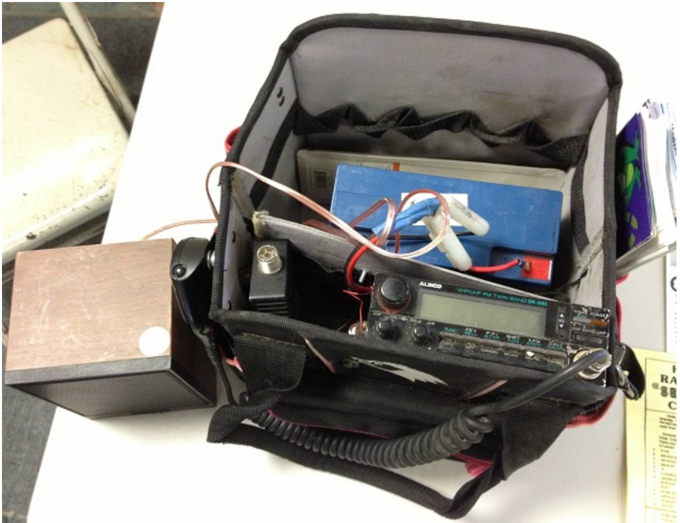
Often seen at CranLand with Ross W1EKG , his Alinco DR-590 VHF/UHF mobile radio, battery and external speaker housed in a square tool bag
