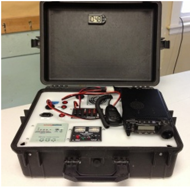
A very nice Yaesu FT-857D based Go-Kit with solar power management and voltage monitoring, assembled by Allen WA1BEE
