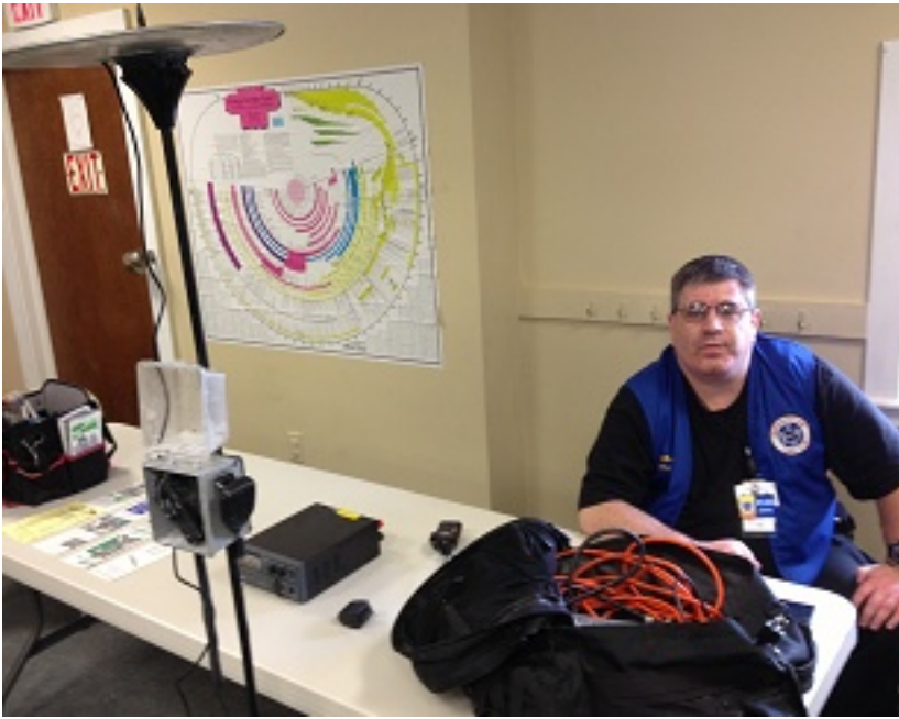
John W1JDG shows his VHF/UHF HT station comprised of a sturdy, cement base, HT enclosure with an external speaker/mic and elevated mag mount antenna with a ground plane base.
