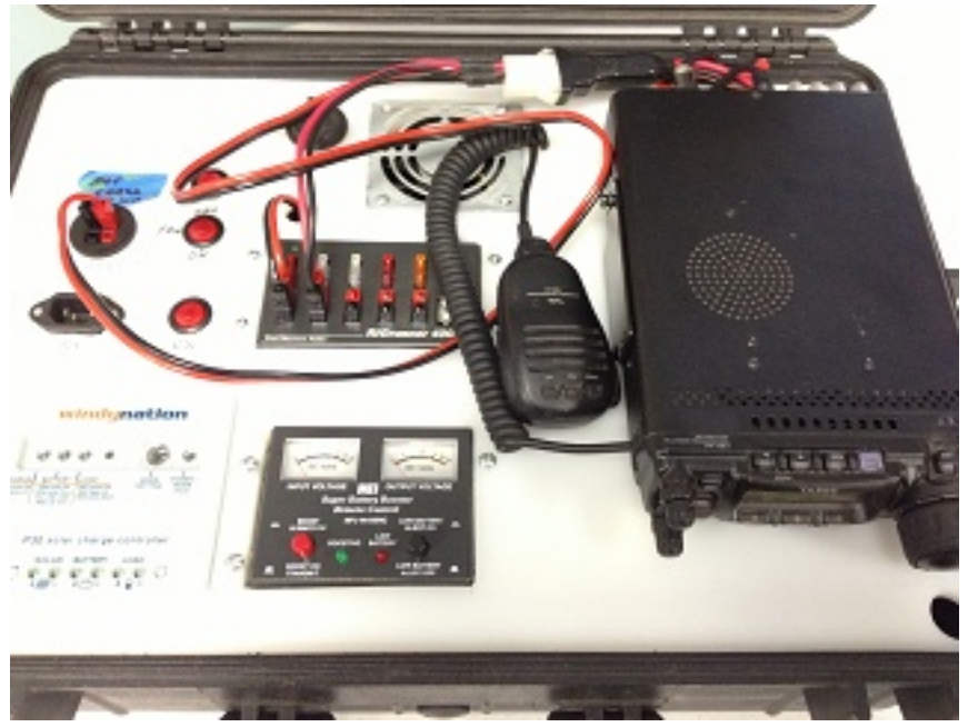
A very nice Yaesu FT-857D based Go-Kit with solar power management and voltage monitoring, assembled by Allen WA1BEE
