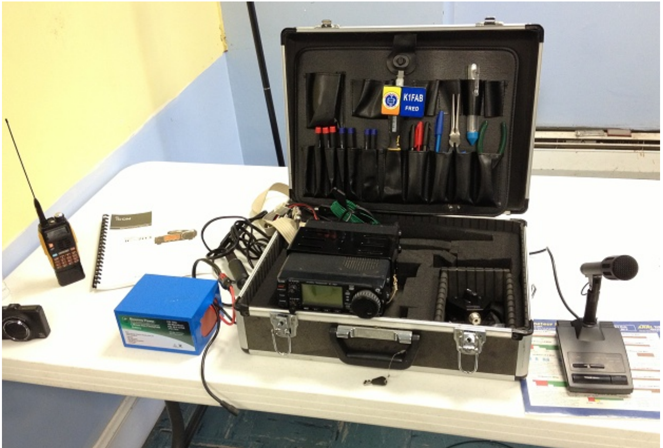
Fred K1FAB showed his Go-Kit featuring an Icom IC-703 QRP HF rig powered by a 12v 15Ah Lithion Iron Phosphate (very light) battery, a Buddy Pole HF antenna and Baofeng HT.
